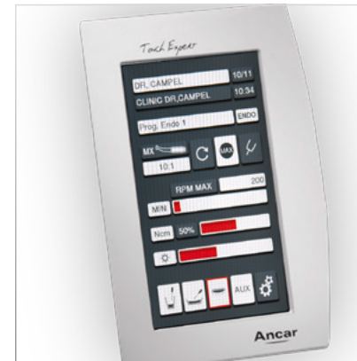
Maximise the performance of your micromotor. Torque control in Ncm, direct or reverse rotation...
